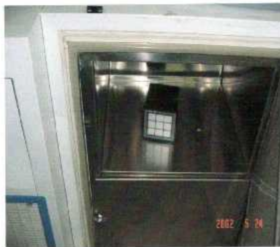
The equipment under cold test
