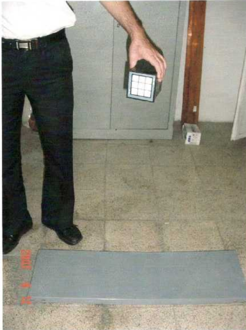
The EUT under the Free Fall test
